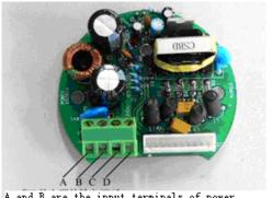
and B are the input terminals of power
